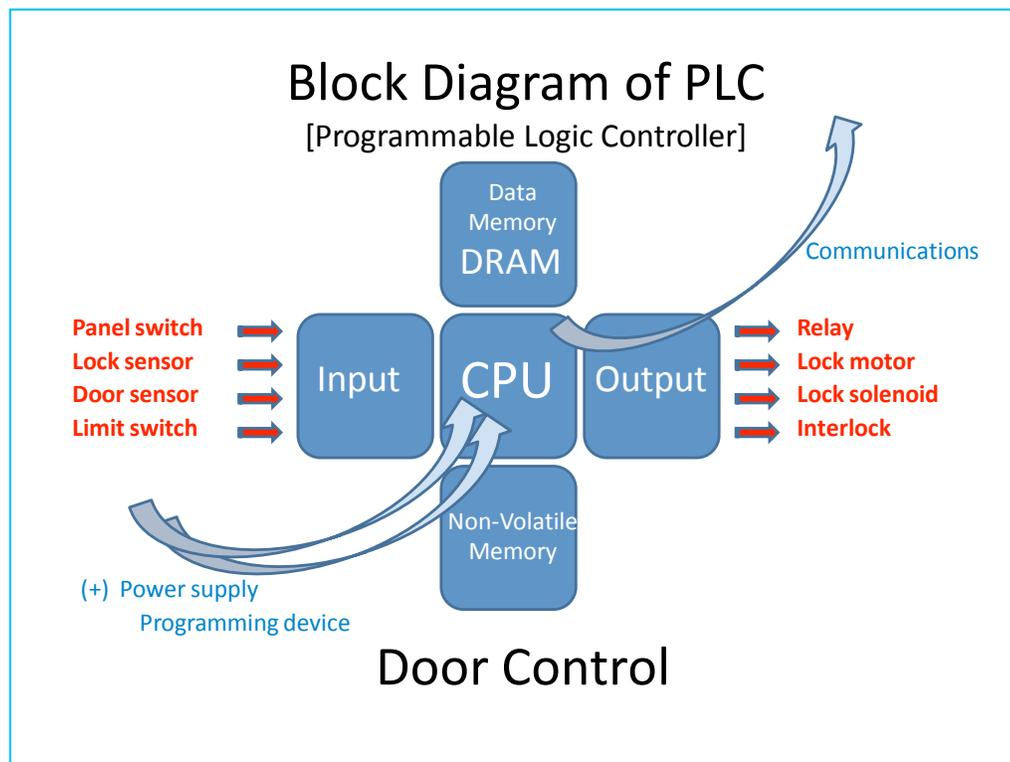
The illustration below (*Figure 2*) is of a pneumatic prison sliding door and dramatizes the fact that, depending upon the sophistication of the door control system, this single door can have as many as 34 points to monitor.
