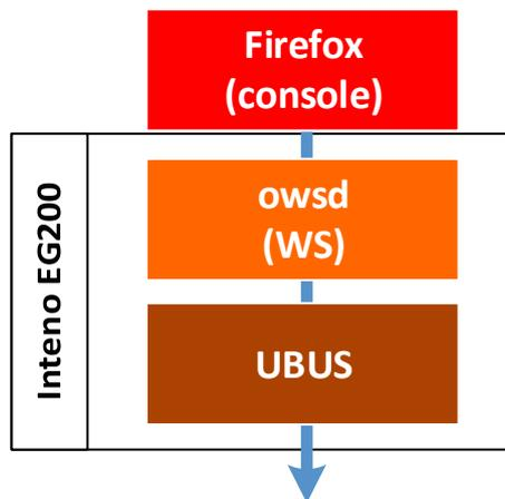
Figure 9: WebSocket communication flow using a browser
