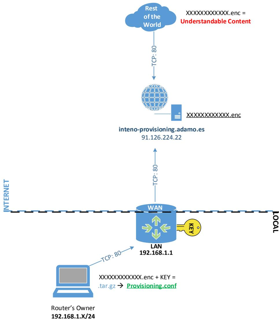
Figure 14: Overview of the hacking process
