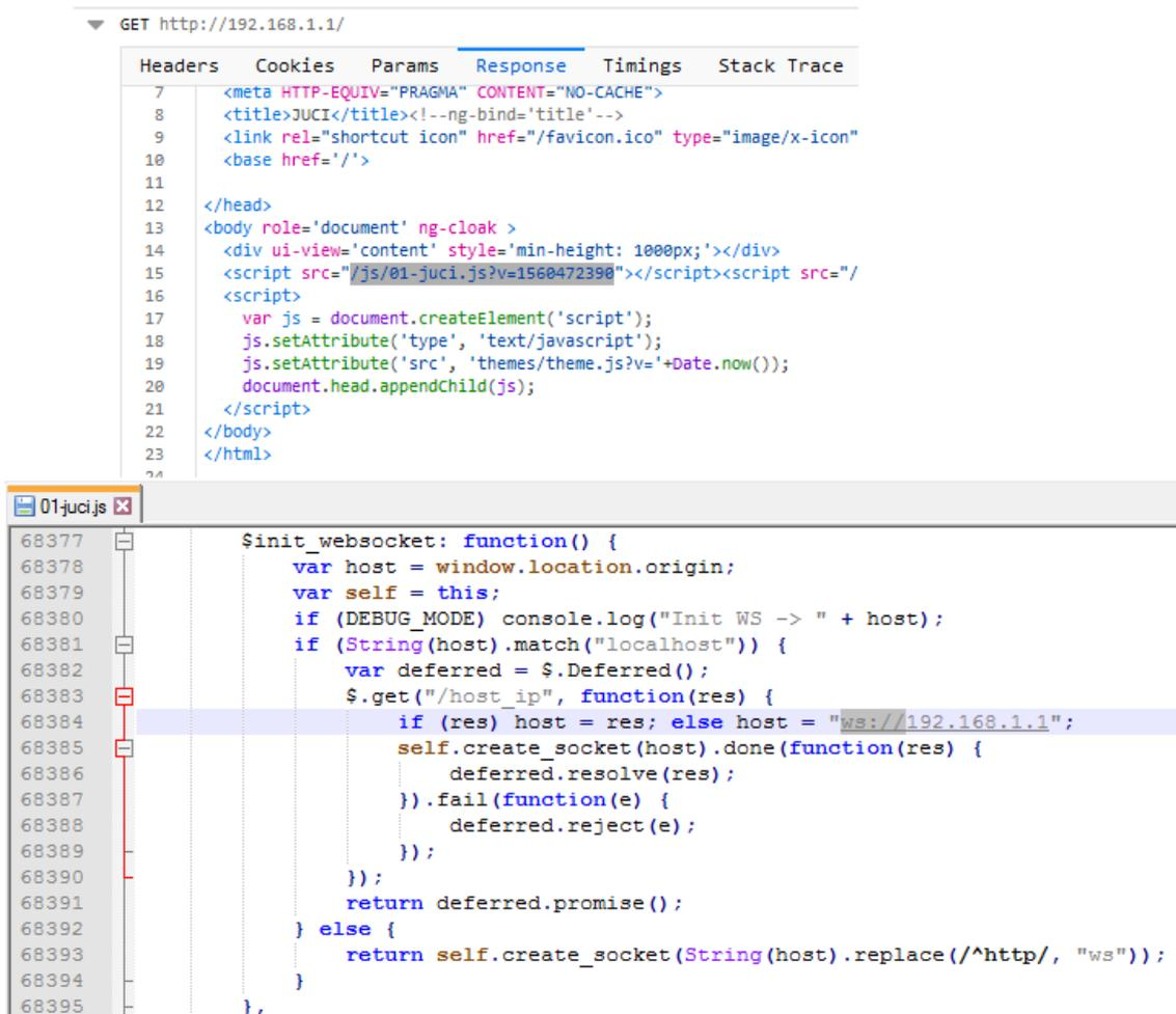
Figure 6: GET request at login's router and script with WebSocket function
