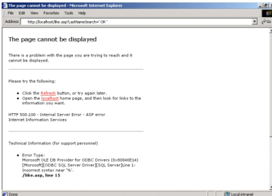
**Figure 3: LIKE breaking on a quoted injection.**
