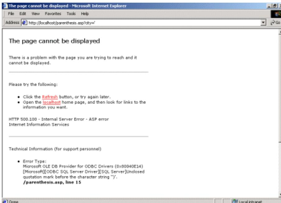
**Figure 2: Parenthesis breaking on a quoted injection.**
