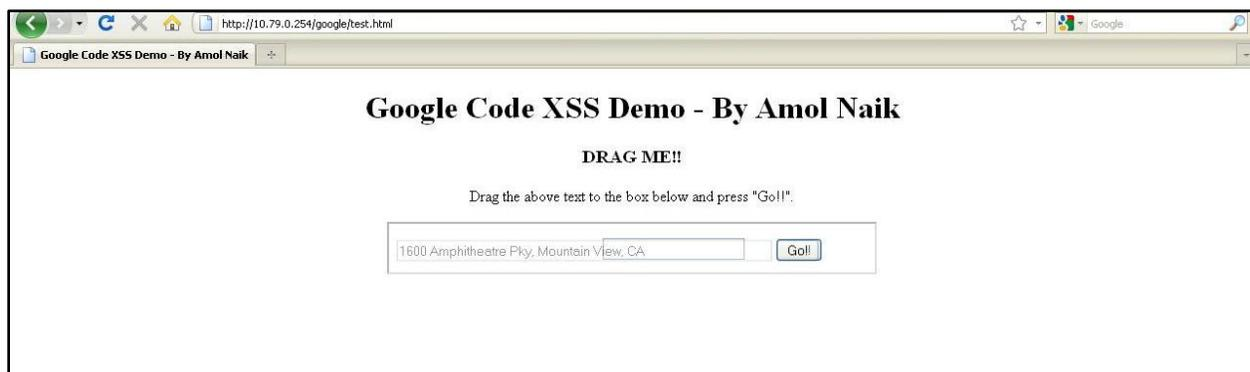
The victim drags the text to input field which holds the XSS payload.
