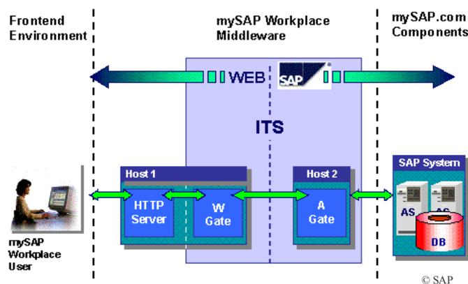
ITS functionality is delivered in the form of *services*. These services are represented by operating system files (*.svc*), located in the Agate server. Each service contains the necessary information to connect to the backend SAP system and perform the required operation.
