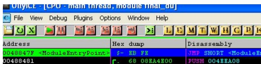
As You can see the first two bytes are EB FE ,they will always trp the program in infinite loop to fix it replace these two bytes with orginal two bytes that are 6A 60
