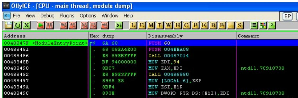
The screenshot shows the OllyICE debugger interface. The CPU window displays the assembly and hex dump of the module entry point at address 0048847F. The assembly code is as follows:
