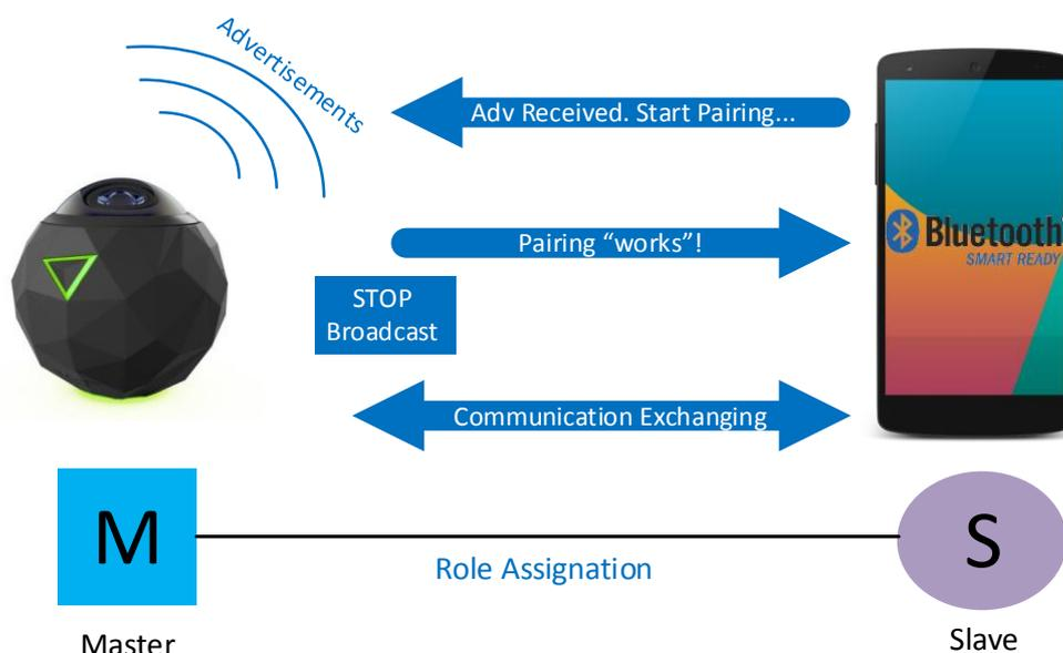
Figure 6: Flow of the connection process and roles assigned
