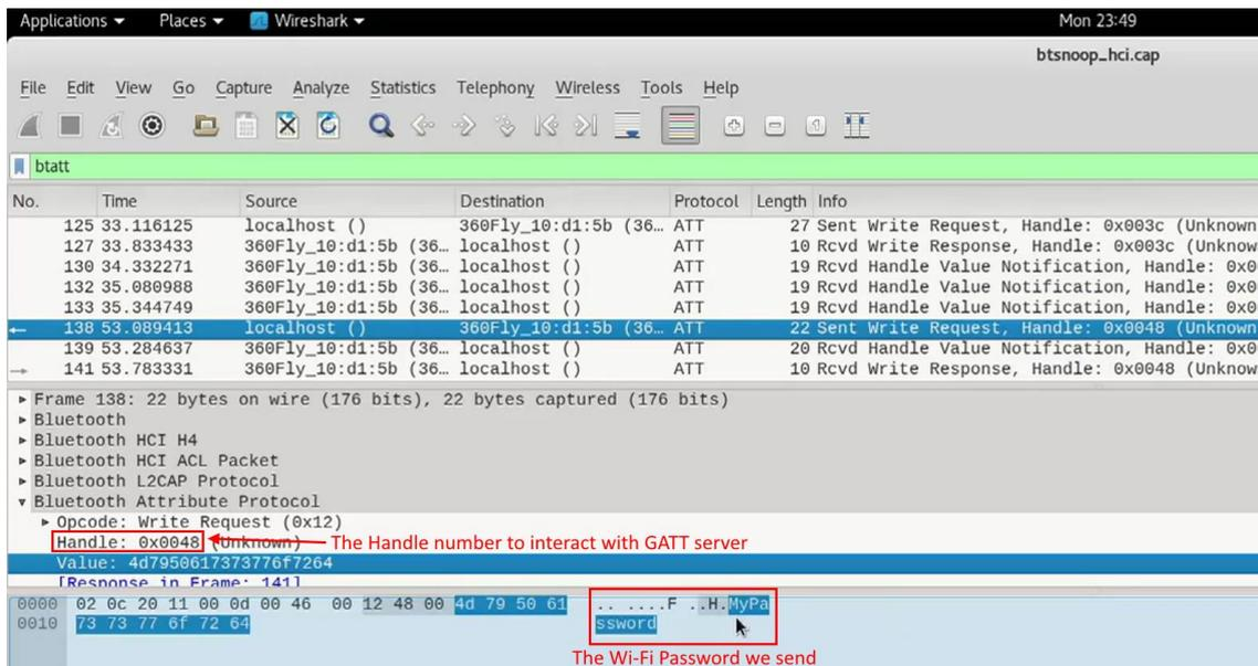
Figure 20: Inspecting BLE packets in Wireshark
