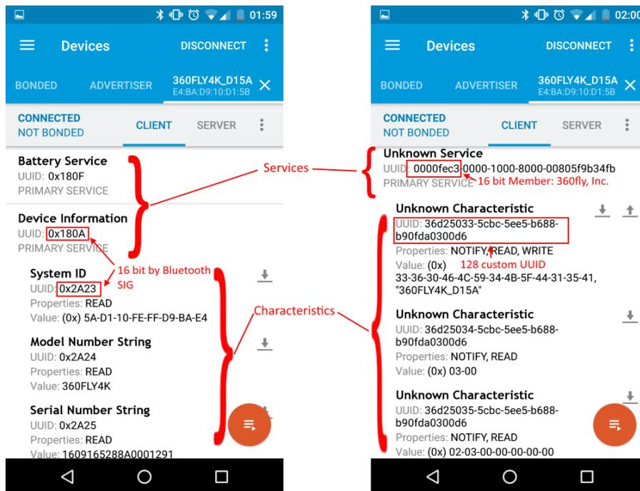
Figure 8: GATT structure on nRF Connect app
