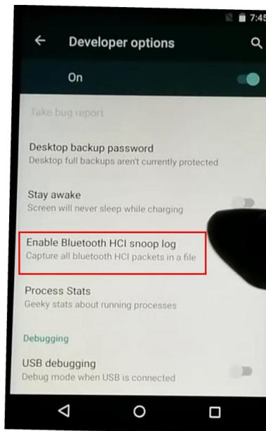
Figure 19: Enabling Bluetooth Sniffing function on Android
