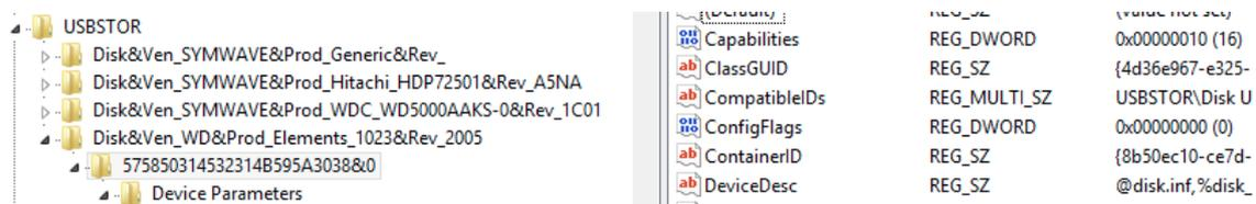
Figure 4: Registry visualization of the USB devices inserted
