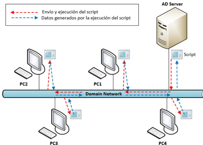
Figure 5: Script release diagram in an AD (Active Directory)
