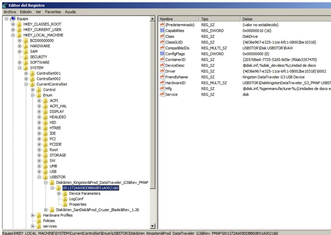
Figure 10: Registry branch where the USB devices are
