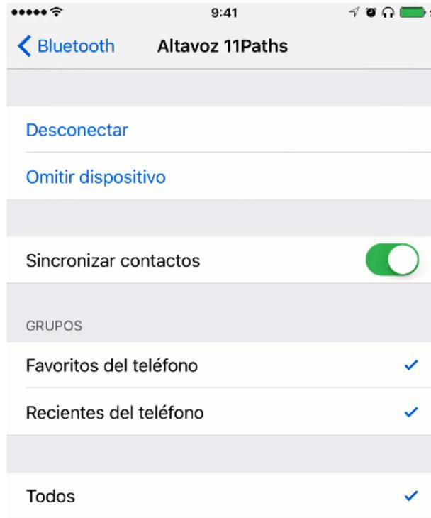
Figure 4: Switch to PBAP profile with automatic contacts synchronization
