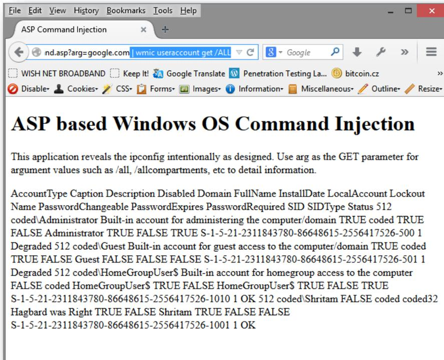
An attacker could also steal 'serial number' of the system to look at the warrantee information. Here I had crafted a payload which could do so: 'google.com | wmic /node:"coded" bios get serialnumber', the string "coded" is in double quote and might need a replacement as per the hostname. The hostname as shown above could be extracted using other system level commands already discussed.
