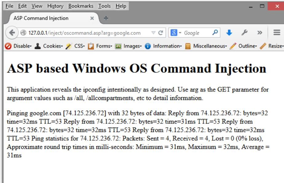
This is normal functionality as designed by the web developer. Common shell commands such as 'dir' on the Windows platform cannot be performed via the URL as shown below since 'ping dir' wouldn't make much sense and will end up treated as a hostname instead with negative results shown:
