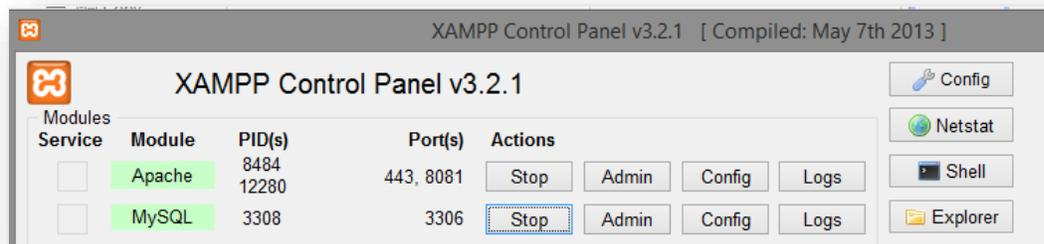
I had configured 'Apache' Web Server to run on port 8081 and 443 instead of port 80 which should be the default. Either way, the application will now be served at port '8081' and to verify this, browse to the 'localhost' with port '8081' or if port '8081' was not setup, the installer has to leave it to default blank as browsers already take port 80 to be the default application web server port.
