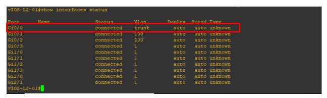
We can see that the interface (G0/0) is set on trunk which means that we can jump other VLANs!
