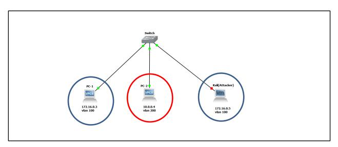
We have the switch which in connected to the PC-1 (IP: 172.16.0.3), PC-2 (IP: 172.16.0.3) and Attacker (IP: 172.16.0.5). The table below explains the clients and the VLAN IDs:
