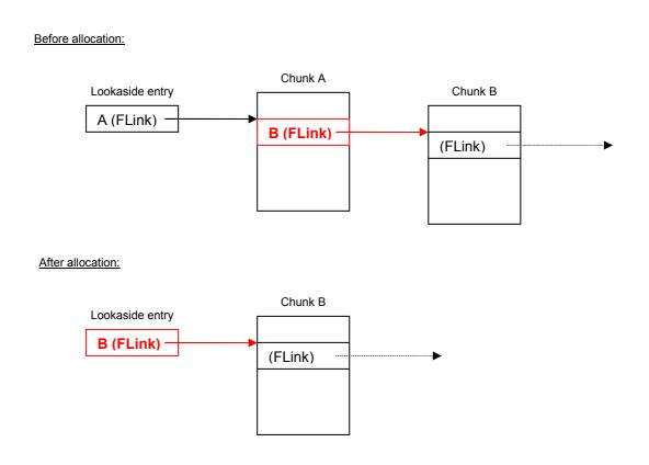
Fig. 1: Allocation of a block A from the lookaside table
