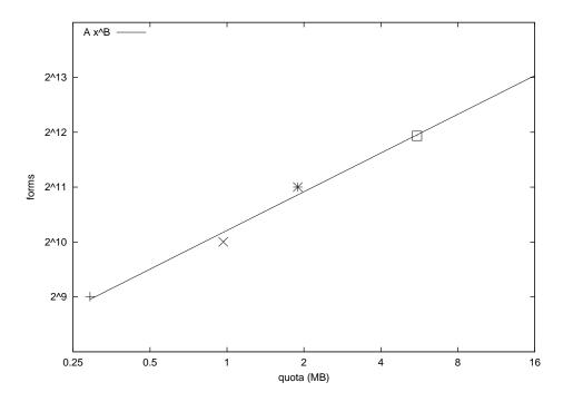
Figure 6: Attack size necessary to kill an account in an hour versus victim's quota. The power law fit yields  $R^2 = 0.9889$ .
