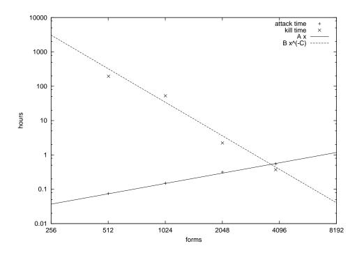
Figure 8: Attack time and time to fill a 2 MB inbox, as a function of attack size. The linear regression for attack time and power law fit for kill time yield  $R^2 = 0.9952$  and 0.977, respectively.
