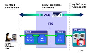
ITS functionality is delivered in the form of *services*. These services are represented by operating system files (*.srvc*), located in the Agate server. Each service contains the necessary information to connect to the backend SAP system and perform the required operation.
