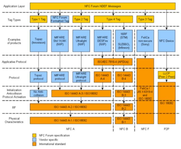
The above figure shows the basic protocol layout of the NFC Stack.
