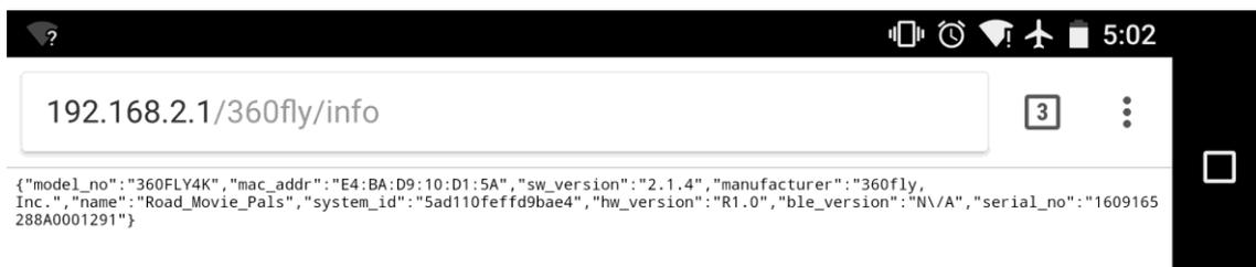
Figure 46: Viewing GET request of ReST in Android
