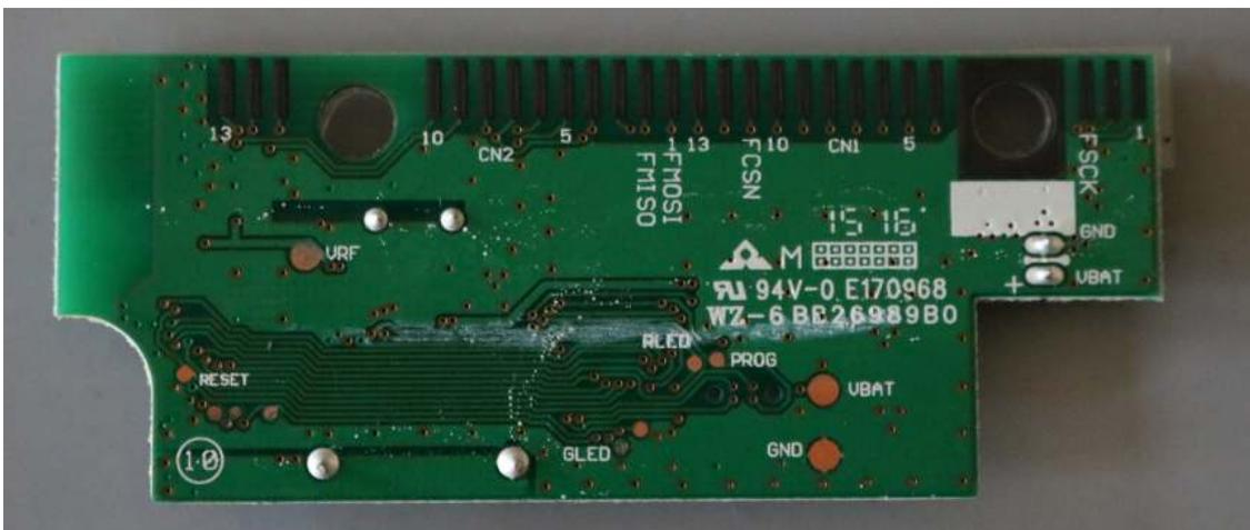
Figure 5: PCB back side of a Microsoft wireless keyboard
