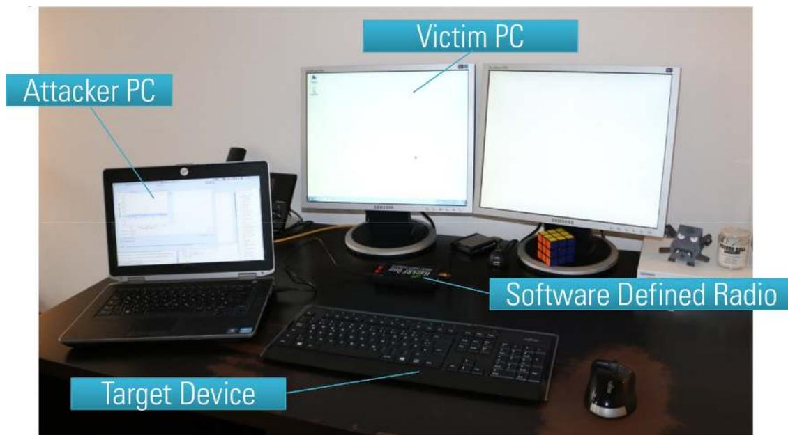
Figure 15: Test setup for simple replay attacks via software defined radio
