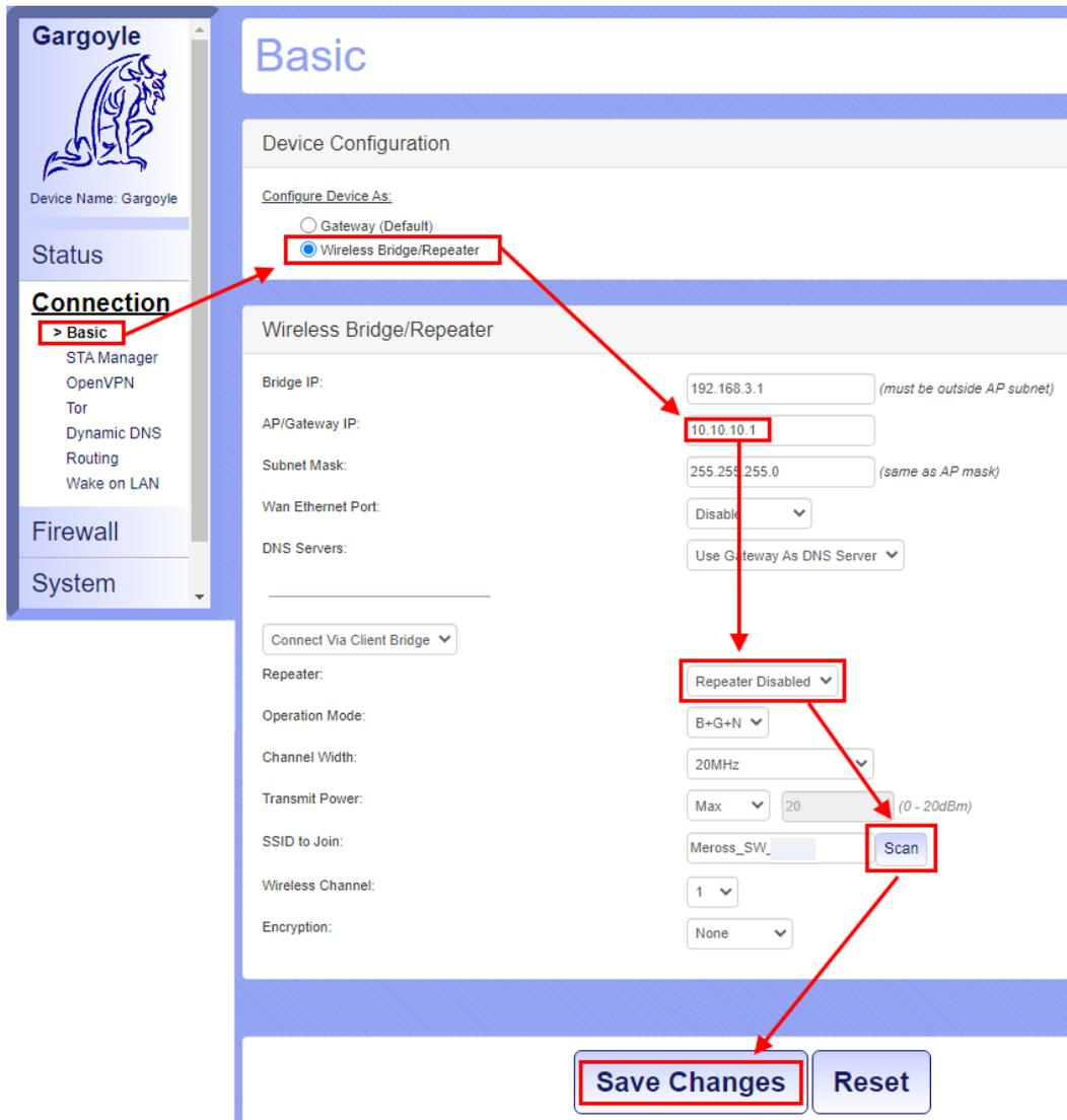
Figure 17: Gargoyle – Set UP the client Wi-Fi mode
